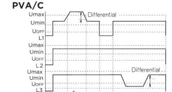
The time delay and differential trip levels help to prevent relay chatter as the monitored voltage level varies.
